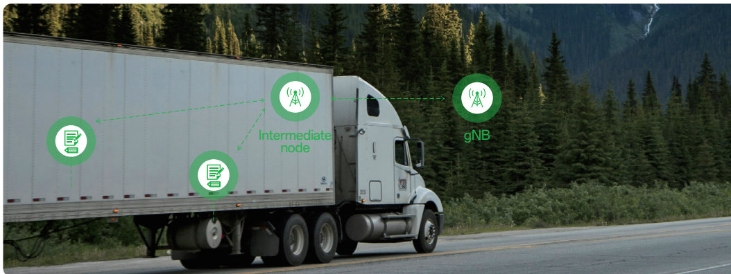
Figure 4.2-5 Relay network topology in cold chain logistics scenario
