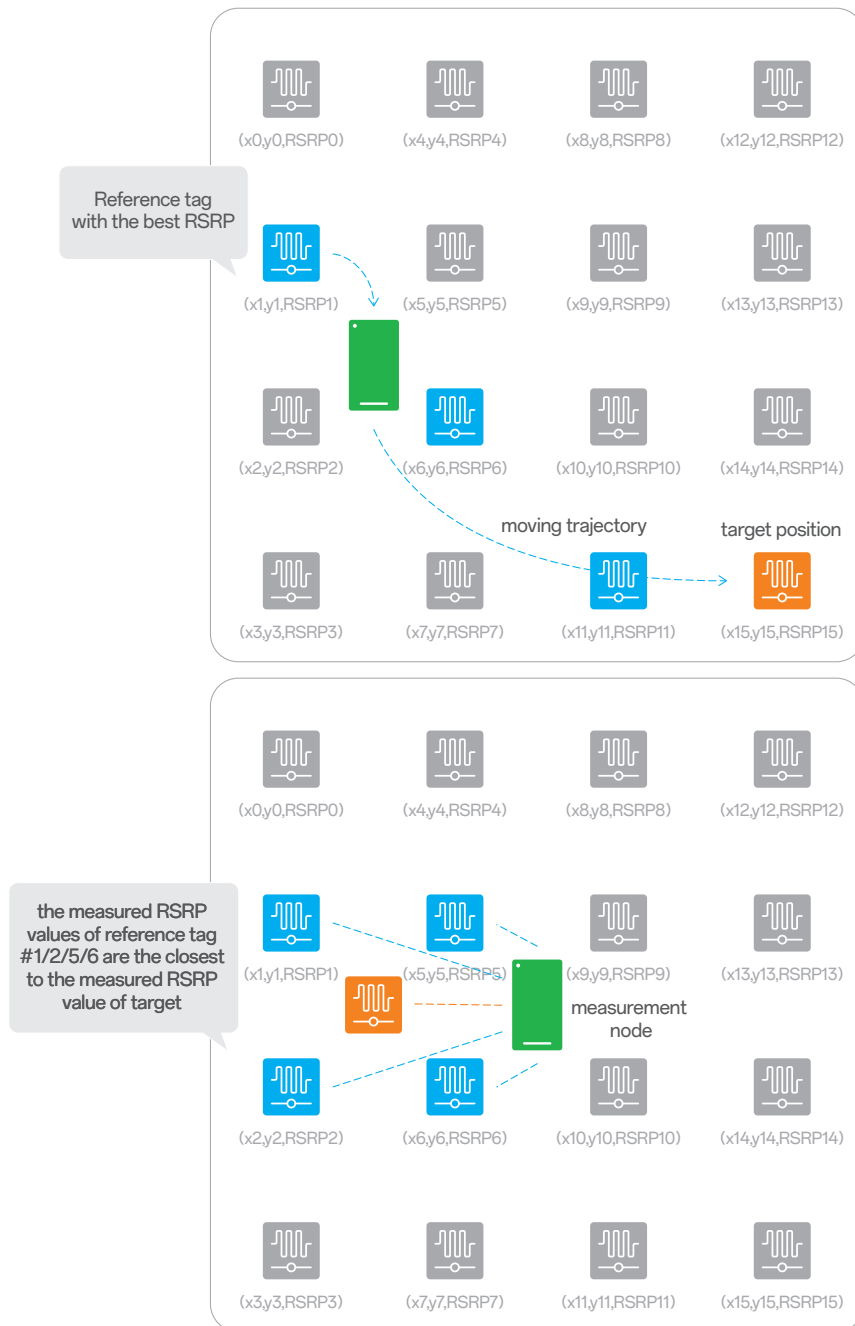
Figure 5.2-2 Signal strength-based positioning method with reference tags
